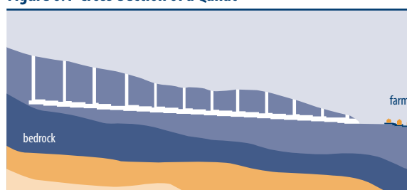
Figure 6.1 Cross-Section of a Qanat
